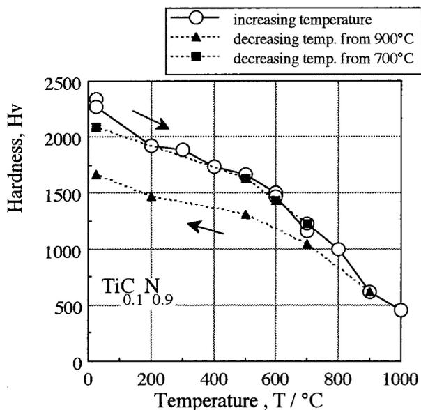
Fig. 5. Hv hysteresis of the Ti–C–N coating. Hv was measured in vacuum at each temperature.
