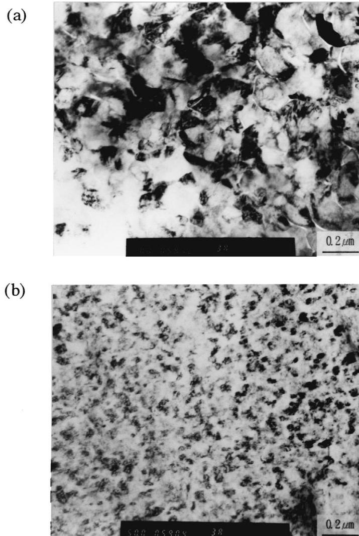
Fig. 8. TEM micrograph of the TiN coating. EB power, 5 kW; substrate temperature, 300°C;  $P_{N_2}$ , 0.05 Pa. (a) Vacuum evaporation, (b) ion plating (substrate current, 3.89 A m<sup>-2</sup>).
