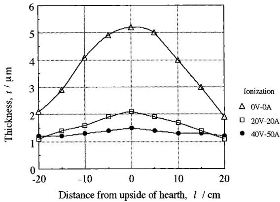
Fig. 9. Effect of ionization on thickness distribution. TiN was deposited at a constant distance of 40 cm from the EB source. Weight of evaporated Ti was 6.0 g.
