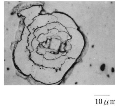
Fig. 3. Self-peeling of TiN deposited at room temperature.
