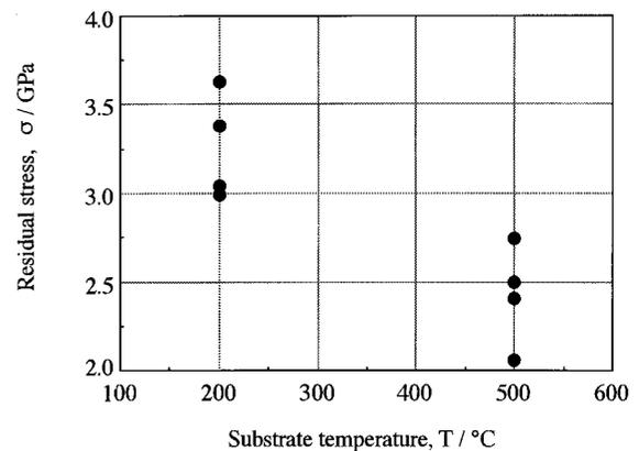
Fig. 4. Effect of substrate temperature on residual stress.
