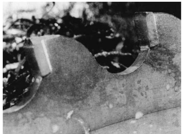
Fig. 12. Ti-C-N-coated tips after cutting 3.4 m<sup>2</sup> of hard steel, showing good adhesion and wear resistance of the coating.
