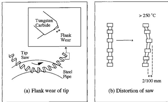
Fig. 2. Tungsten carbide-tipped saw.
