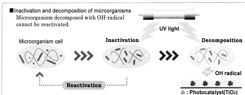
**Fig. 2 Schematic presentation of the disinfection mechanisms by TiO<sub>2</sub>/UV system**
