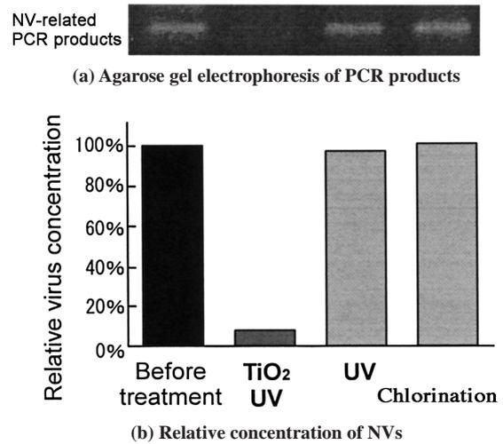
Fig. 8 Comparison of decomposing efficacy of TiO<sub>2</sub>/UV, UV or chlorination
