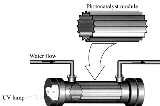
Fig. 4 Example of  $\text{TiO}_2/\text{UV}$  irradiation apparatus
