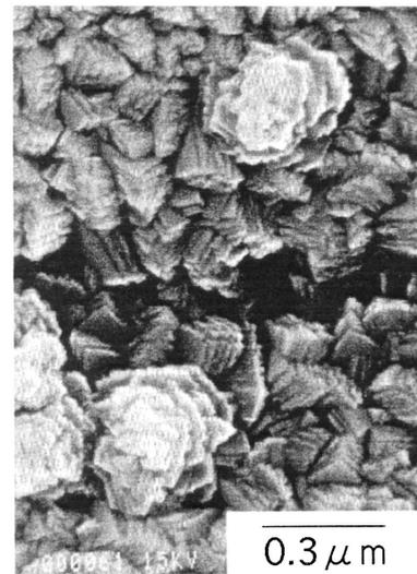
**Fig. 3 Scanning electron microscopic photograph of the newly developed photocatalyst**
