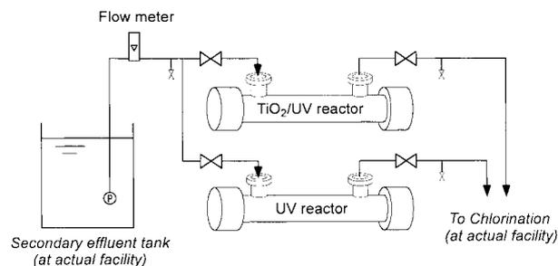
Fig. 5 Experimental flow diagram
